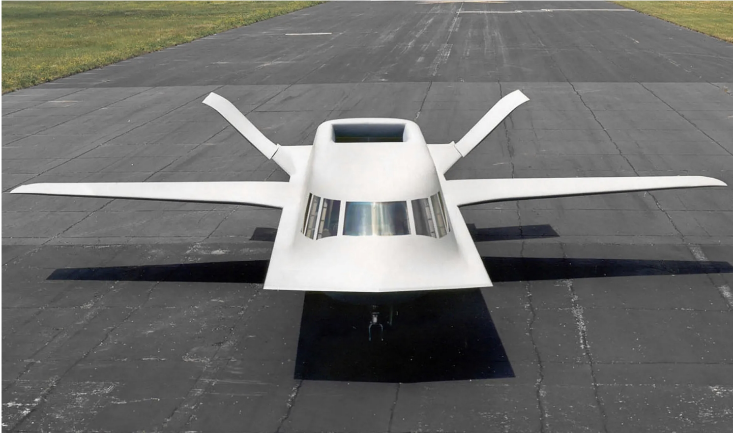
Figure 14: Image of Tacit Blue: "The advancements in stealth technology made with the Tacit Blue can still be observed in the lineage of the B-2 and B-21, as the setup and angle of the cockpit windows is a clear evolution of the Tacit Blue's design"
